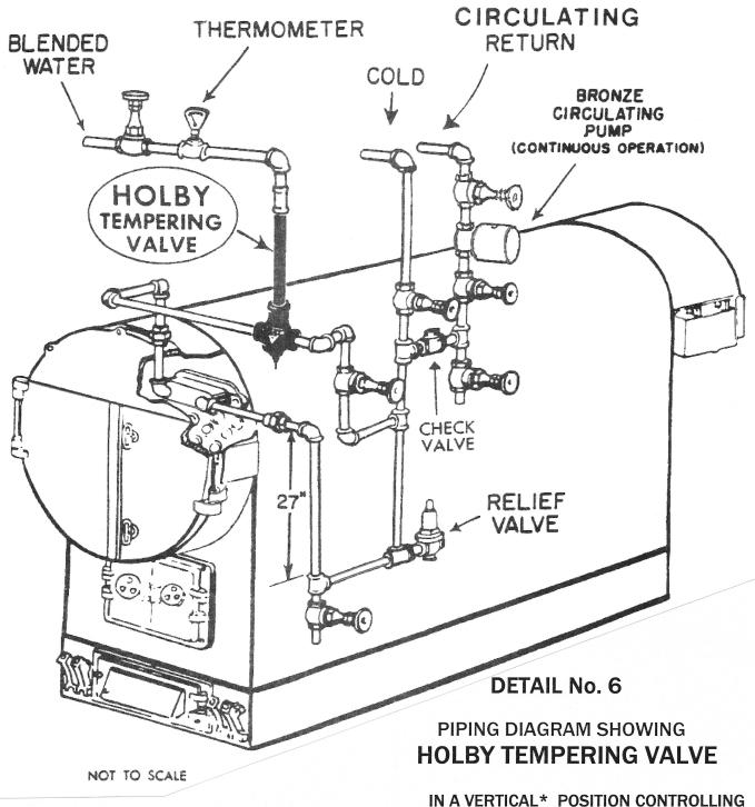
IN A VERTICAL\* POSITION CONTROLLING THE TEMPERATURE OF HOT WATER DELIVERED BY A SUBMERGED TANKLESS WATER HEATER.
