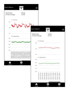
The HolbyMonitor App provides simple temperature graphs of hot water and mixed water. Select various reports from 2 hours to 7 days as well as a custom date range.
